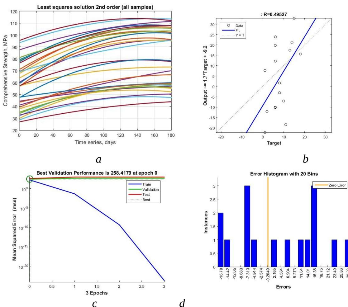
Fig. 2. Data of performing prediction of the concrete strength: a – Last Squares Solution 2<sup>nd</sup> order for all samples; b – Regression; c – Best Validation Performance; d – Error Histogram;
