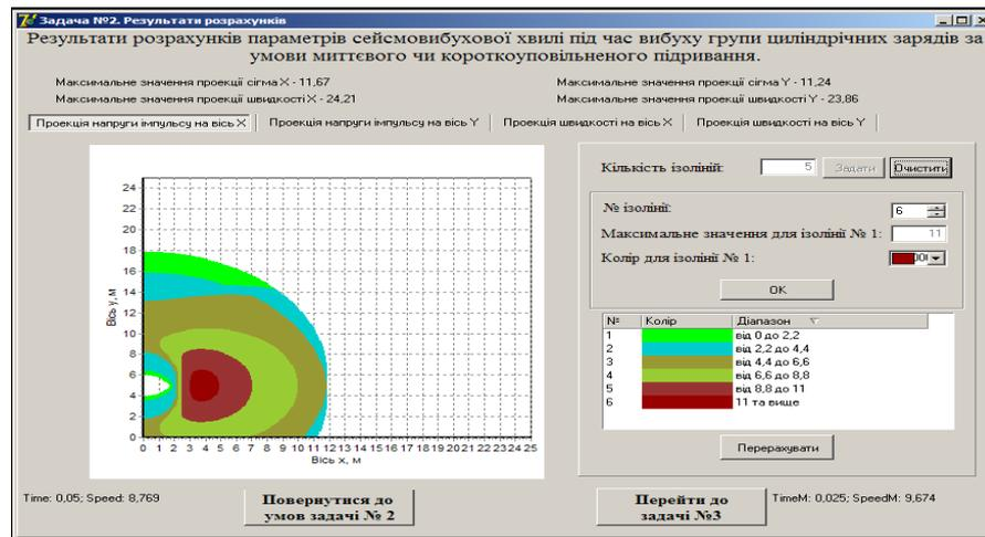
Fig. 4. The output window of the results for the task about the explosion of cylindrical charge group in soil massif
