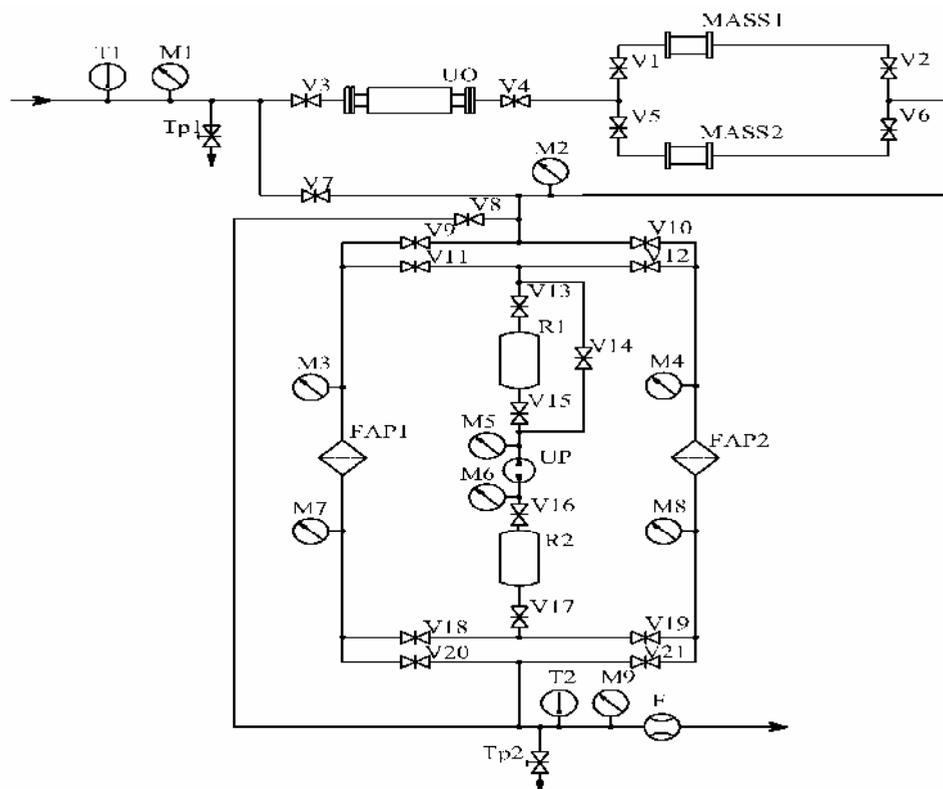
Fig. 2. Hydraulic circuit of ultrasonic magnetic adsorptive system of water purification
