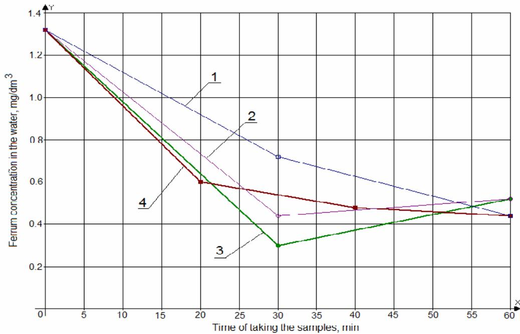
Fig. 3. The ferrum concentration in the water under the action of various units of UMASWP: 1 – MASS and UO; 2 – FAP1; 3 – MASS, UO, FAP2; 4 – MASS, UO, FAP1
