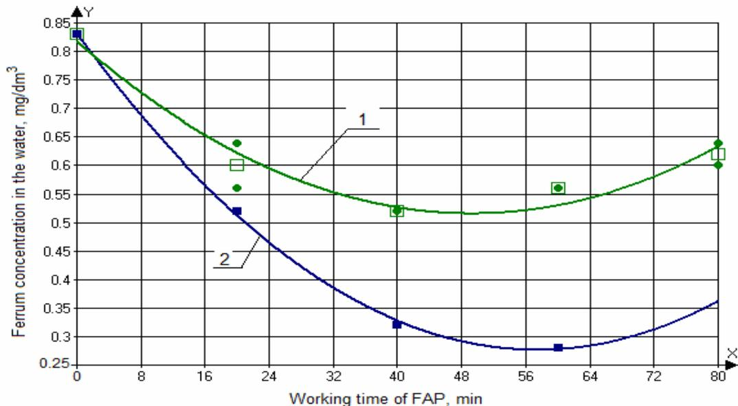
Fig. 4. The ferrum concentration in the water according to the action period of UMASWP: 1 – UMASWP without regeneration of FAP; 2 – UMASWP after regeneration of FAP
